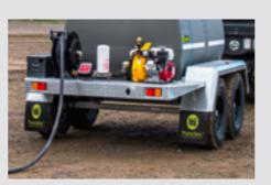
65MM 4T-RATED GALVANISED AXLES WITH 15" LANDCRUISER WHEELS
