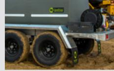
**HEAVY DUTY HOT-DIP GALVANISED STEEL CHASSIS**
